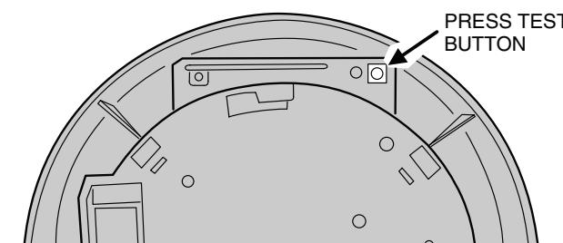
**STEP 7 Attach TSD-90A to mounting plate.** Match up alignment tabs on alarm and plate. Turn alarm clockwise until it locks in place (tamper switch will click as alarm locks onto plate).
